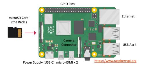
Figure 1.3: Raspberry Pi Connectors
