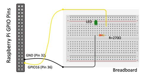
Figure 1.9: LED wiring
