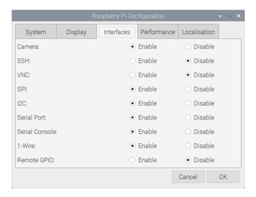
Figure 1.11: Enable/Disable Raspberry Pi Hardware Interfaces
