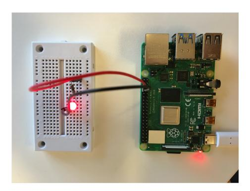
Figure 1.10: LED wiring
